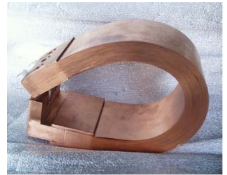
Copper wire and terminal welded together to improve the resistance
