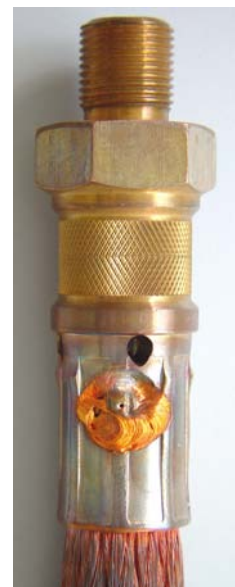
Copper wire and terminal welded together to improve the resistance
