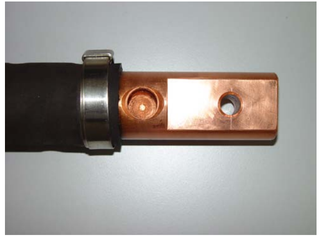
700 mm 2 water-cooled welding cable with flat terminals
